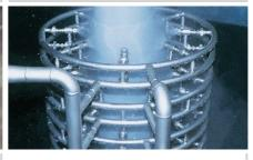
Ring header equipped with pneumatic nozzles. providing uniform spray from all directions.
