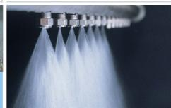
Spray header with MOMOJet®, purging foreign particles by reducing the pressure.
