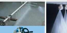
Spray header with inner brush, which clears the clog by turning a handwheel
