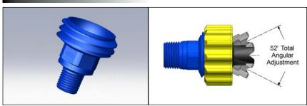
The BEX threaded K-Ball® body provides the ability to adjust the direction of the spray pattern by simply twisting the K-Ball® cap, repositioning the nozzle and tightening the cap. The same 52°nozzle angle of adjustability exists in the threaded body as in the K-Ball®
