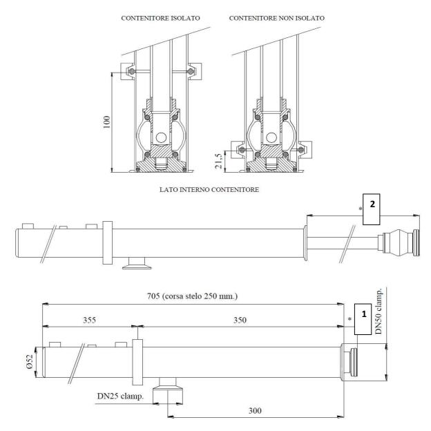
The weight of a head rotating about an axis varies from 3.40 to 3.70 Kg depending on the model
