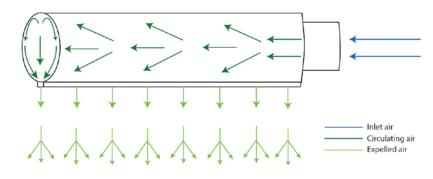
An air knife is a pressurized air plenum with a uniform continuous gap which pressurized air exits in a laminar flow pattern. The exiting air velocity creates an impact air velocity directly onto the surface of the product to shear away moisture or particulates without mechanical contact. This impact air velocity can range from a gentle breeze to greater than 40,000 feet per minute.
